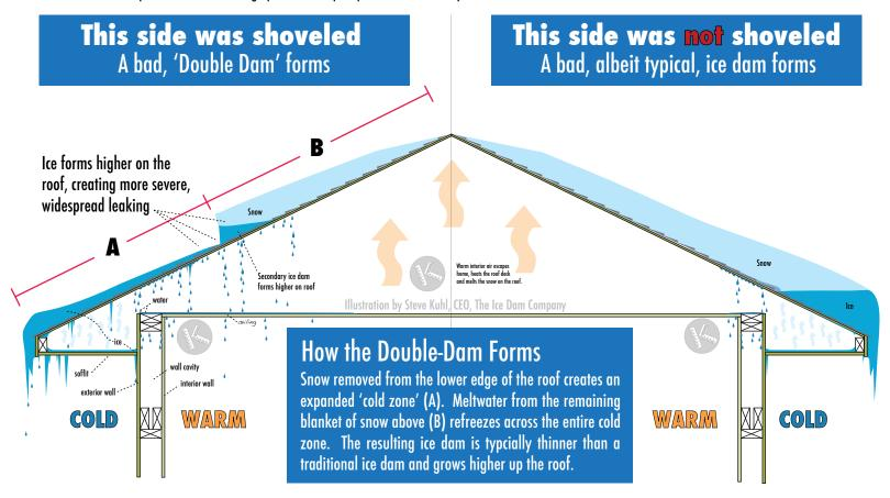
Of the two ice dams illustrated above, the Double Dam presents a couple of challenges beyond those of the regular ice dam. First, because ice has grown further up the roof slope, the subsequent leaks inside will cover a wider area. The second problem with a Double Dam is the cost of removal. Although half the thicknessmay take two to three times longer to remove than a regular ice dam. More time equals more money.
